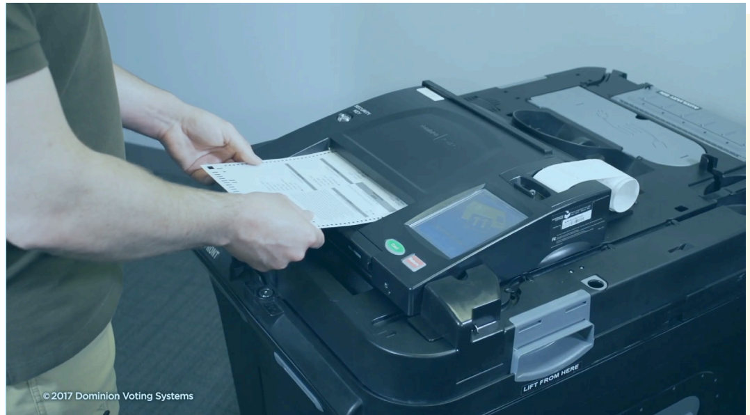
Figure 2. A voter inserts a ballot into the Dominion ImageCast Precinct, which scans and tabulates the ballot. (Source: Dominion Voting Systems / YouTube) 16
