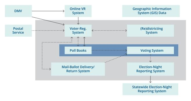
Arrows depict the direction of information flow between component systems. Solid lines indicate flows that typically rely on the Internet or other networks that are connected to the Internet; dashed lines indicate information flows that typically are "air-locked" from outside networks. The dark blue box indicates systems that are typically deployed in individual polling places; the grey box indicates systems that are typically centralized in a local jurisdiction's election office.
